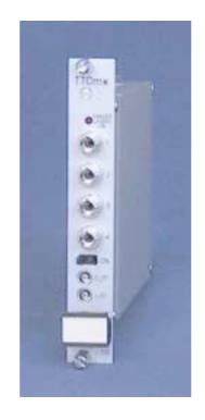
Fig. 10 TTCmx laser transmitter
