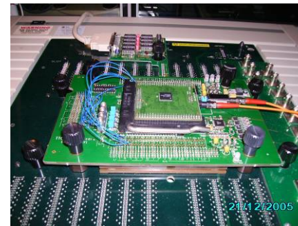
TTCrq tester EDA-00975-V1 Mounted on the IC tester (PH/MIC). Used to test 2200 TTCrq in 4 different configurations
