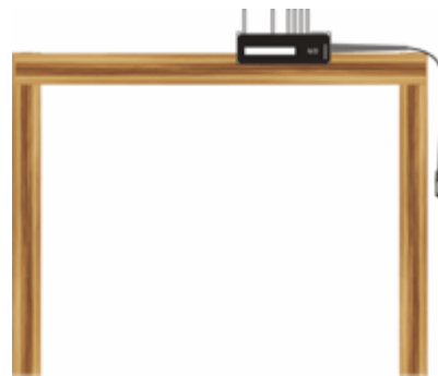
Figure 2: Letting the Fiber Dangle Over Sharp Corners will Damage the Fiber
